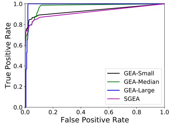
Fig. 13: DL-FHMC: RF-based suspicious behavior detector ROC performance over GEA and SGEA attacks.
