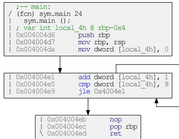
Fig. 1: The generated CFG for the original sample and used for extracting graph-based features (graph size, centralities, *etc.*) for graph/program classification and malware detection.
