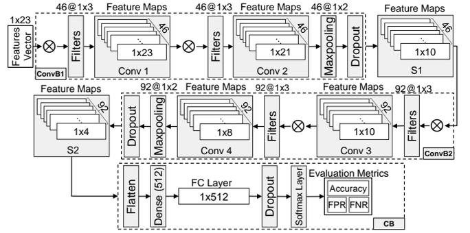
Fig. 7: Internal design of the CNN architecture used for detection and classification task. Notice that  $46@1 \times 3$ , for example, refers to applying 46 filters each of size  $1 \times 3$  on the input data. The design consists of four convolutional layers with maxpooling and dropout operations. Then, a dense layer of size 512 is used with a softmax activation function to output the model's prediction.
